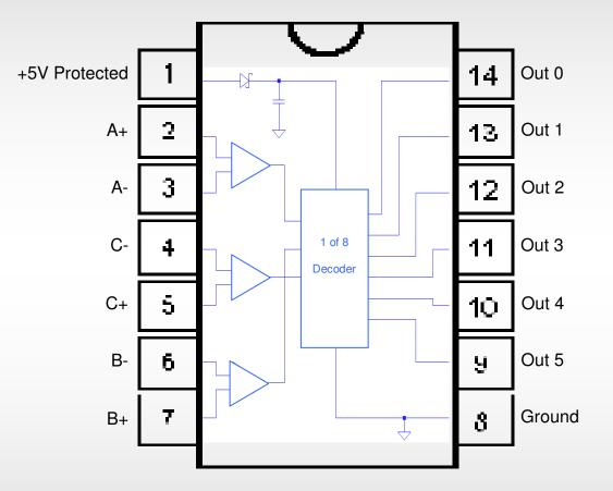
Three line receivers accept complementary logic over a +/-7V range, with a sensitivity of 200 mV and a built-in 50mV hysteresis for clean switching in noisy environments. This provides RS-422 compatibility, as well as compatibility with a wide range of balanced logic formats.
